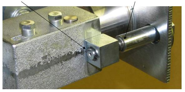
6. TO VERIFY THE UNIT IS INSERTED CORRECTLY AND READY FOR USE MAKE SURE THE OPENING PIN IS DEPRESSED INTO THE OPENING PIN BONNETT. SEE PHOTO BELOW
